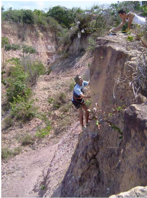
Figure 2a: Soil sample collection using a rope technique on Araçagi gully wall.
