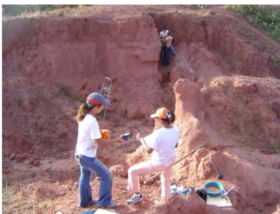
Figure 2c: Soil sample collection and GPS measurement, at COEDUC gully.
