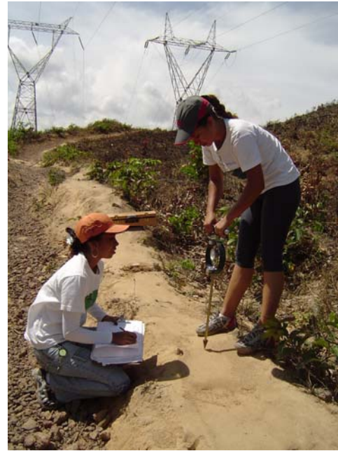
Figure 2b: Use of the penetrometer on a track around Bacanga gully.
