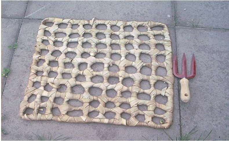
Plate 2: Palm mat geotextile
